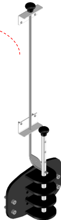
Manual uncoupling lever in the driver compartment (coupling attachment)
