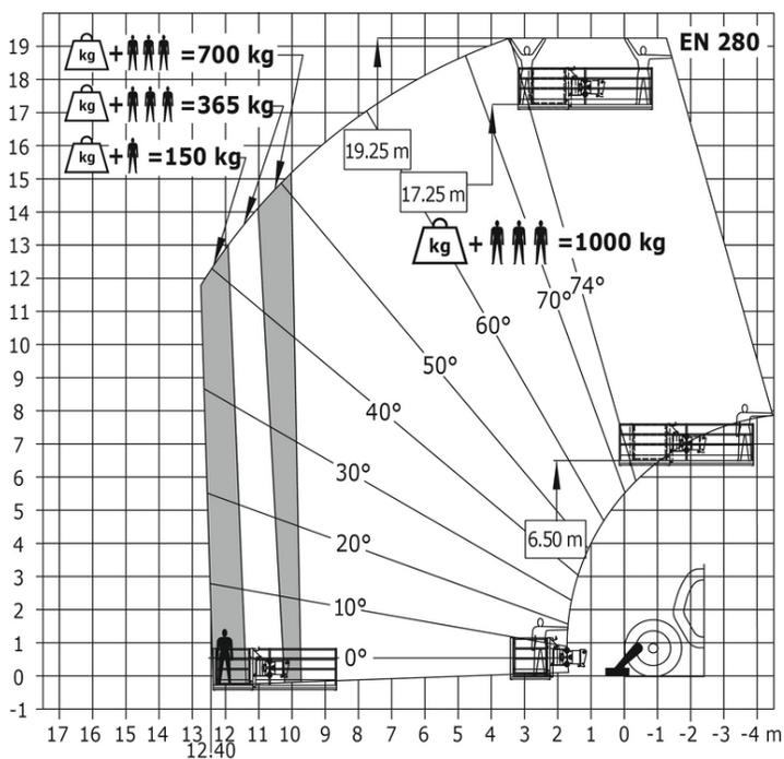
Machine on tyres with forks - with levelling Metric
